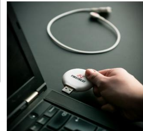
4 The measurement starts automatically when the device is attached. Make sure the green light is blinking. Note! The light is easiest to see in the dark.
