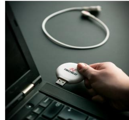
4 The measurement starts automatically when the device is attached. Make sure the green light is blinking. Note! The light is easiest to see in the dark.
